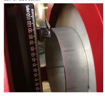
Tube with small diameters <25.4 mm are particularly concerned by the facing process. They are often cut with tube cutters or abrasive cutting machines. Generally speaking, tube must be faced before welding in order to obtain quality welds.
